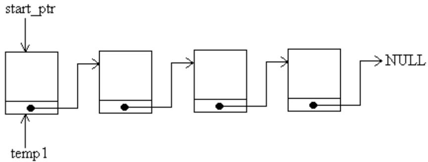
The **next** pointer from this node isn't NULL, so we haven't found the end node. Instead, we set the pointer **temp2** to the same node as **temp1**
