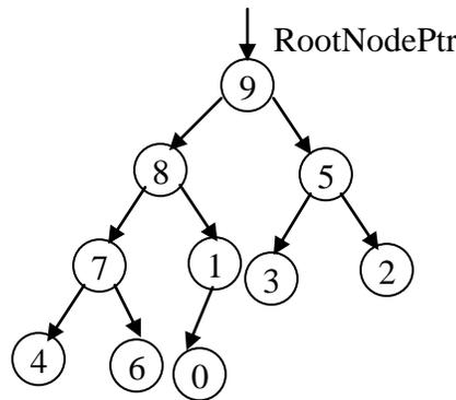
Swap the root node with the lowest, right most node and delete the lowest, right most value; insert the deleted value in the array in its proper position; adjust the heap tree; and repeat this process until the tree is empty.
