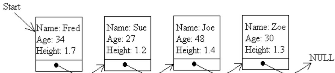
This linked list has four nodes in it, each with a link to the next node in the series. The last node has a link to the special value NULL, which any pointer (whatever its type) can point to, to show that it is the last link in the chain. There is also another special pointer, called Start (also called head), which points to the first link in the chain so that we can keep track of it.
