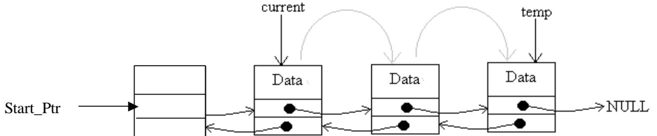
After that, a new node is declared, and the name is copied into it. The `nxt` pointer of this new node is set to `NULL` to indicate that this node will be the new end of the list. The `prv` pointer of the new node is linked into the last node of the existing list. The `nxt` pointer of the current end of the list is set to the new node.
