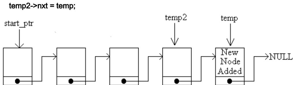
The link **temp2->nxt** in this diagram is the link joining the last two nodes. The full code for adding a node at the end of the list is shown below, in its own little function:
