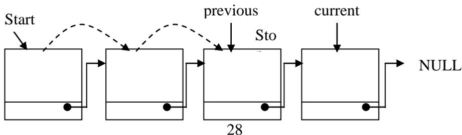
First of all, we had better check to see if the current node is also first the one. If it is, then there is no "previous" node to point to. If not, check through all the nodes in turn until we detect that we are just behind the current one (Like a pantomime - "behind you!")
