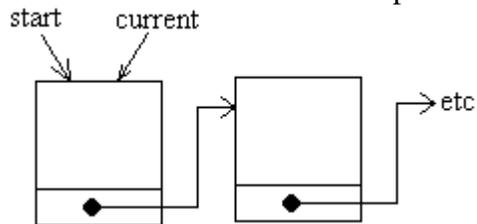
It's easy to get the **current** pointer to point to the next node in the list (i.e. move from left to right along the list). If you want to move **current** along one node, use the **nxt** field of the node that it is pointing to at the moment:
