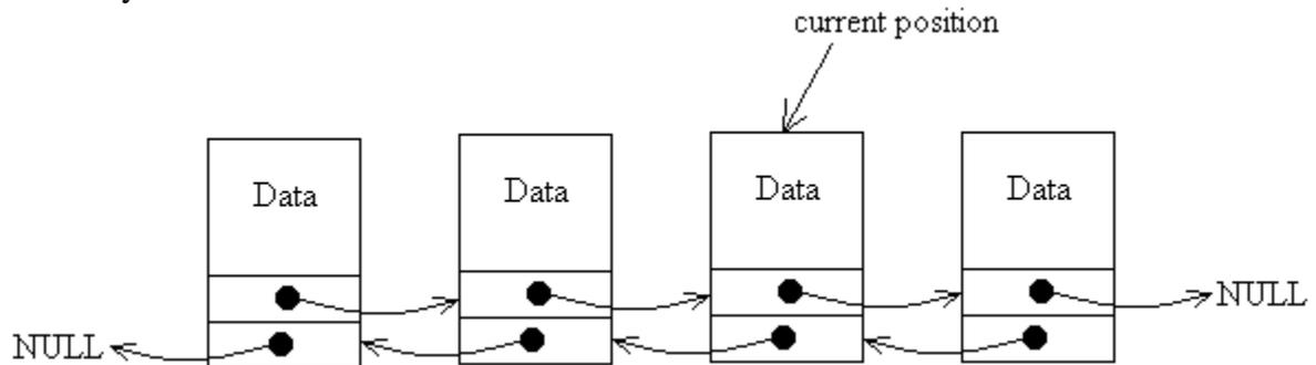
You will notice that each node in the list has two pointers, one to the next node and one to the previous one - again, the ends of the list are defined by NULL pointers. Also there is no pointer to the start of the list. Instead, there is simply a pointer to some position in the list that can be moved left or right.
