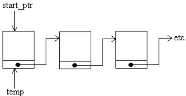
Now that the first node has been safely tagged (so that we can refer to it even when the start pointer has been reassigned), we can move the start pointer to the next node in the chain:
