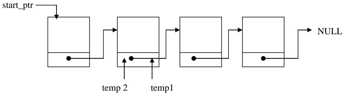
and **temp1** is made to point to the next node along:
