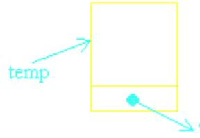
We can refer to the new node as `*temp`, i.e. "the node that `temp` points to". When the fields of this structure are referred to, brackets can be put round the `*temp` part, as otherwise the compiler will think we are trying to refer to the fields of the pointer. Alternatively, we can use the arrow pointer notation.
