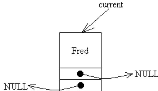
We still need to consider the directions 'forward' and 'backward', so in this case, we will need to define functions to add a node to the start of the list (left-most position) and the end of the list (right-most position).
