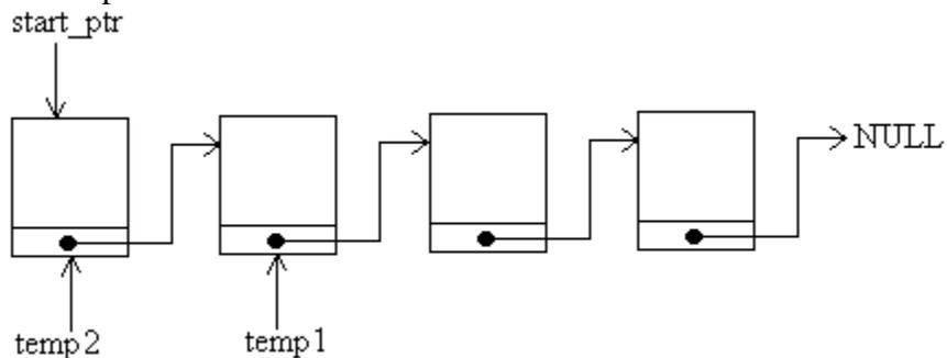
Going back to step 3, we see that temp1 still doesn't point to the last node in the list, so we make temp2 point to what temp1 points to
