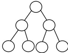
Complete binary tree: a binary tree in which the length from the root to any leaf node is either  $h$  or  $h-1$  where  $h$  is the height of the tree. The deepest level should also be filled from left to right.
