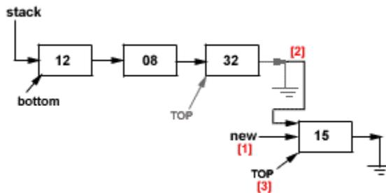
In Step [1] we create the new element to be pushed to the Stack.
