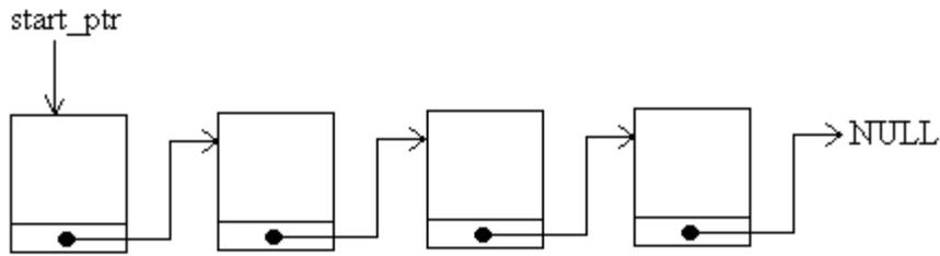
Firstly, the start pointer doesn't point to NULL, so we don't have to display a "Empty list, wise guy!" message. Let's get straight on with step2 - set the pointer **temp1** to the same as the start pointer:
